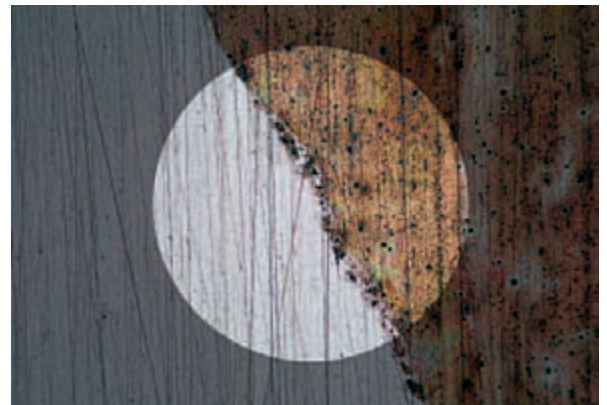
Fig 3: Under the microscope at x100 the region protected by the plasma layer (left) exhibits no sign of corrosion even after direct exposure to the salt spray test for 96 hours.
