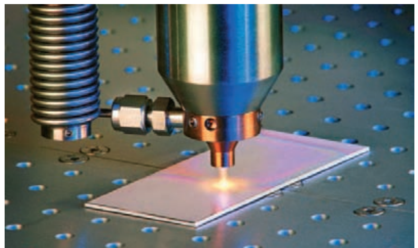
Right: Open-air-PlasmaPlus for nanocoating of surfaces
