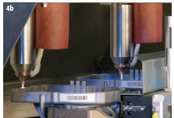
Figs 4a & b: Prior to plasma coating the motor housings are precleaned with the atmospheric-pressure plasma (4a) after which they are coated with a monolayer film by adding a precursor material to the plasma (4b)
