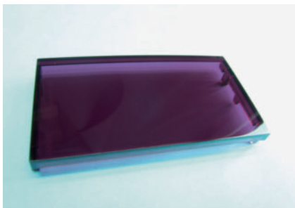
Fig. 6. Following microscopic cleaning and intense activation by plasma radiation, the plastics are given their scratch-proof coating in the varnishing unit (photo: GfO)
