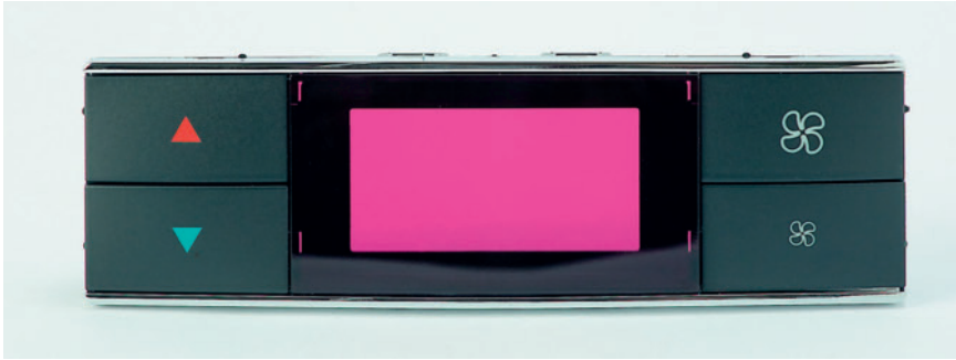
Fig. 3. Colored display fascia for air conditioning system. Treating the panes with plasma at atmospheric pressure leads to spotless optics and optimum adhesion of the scratch-proof coating
