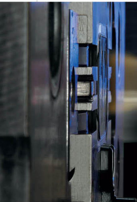
Fig. 5. View into the injection moulding machine: The Openair plasma beam impinges with almost ultrasonic speed on the polycarbonate lenses. Microfine cleaning and strong activation impart new adhesion properties to the plastic material
