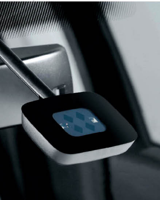
Fig. 1. The highly complex polycarbonate optics of the sensors is manufactured in a three-component injection moulding process (figures: Plasmatreat)
