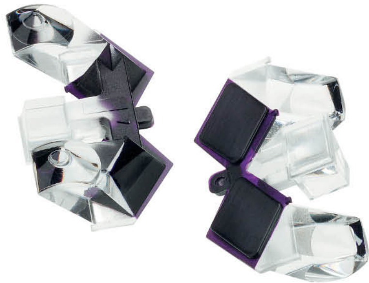
Fig. 1. The highly complex polycarbonate optics of the sensors is manufactured in a three-component injection moulding process (figures: Plasmatreat)
