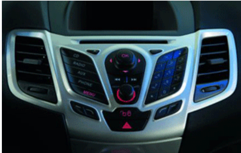
Fig.5. Photo Plasmatreat The integrated control panel (ICP) forms the centrepiece of the dashboard. The plastic switches are pretreated with atmospheric plasma before painting to ensure a flawless finish and an adhesion that will last for years
