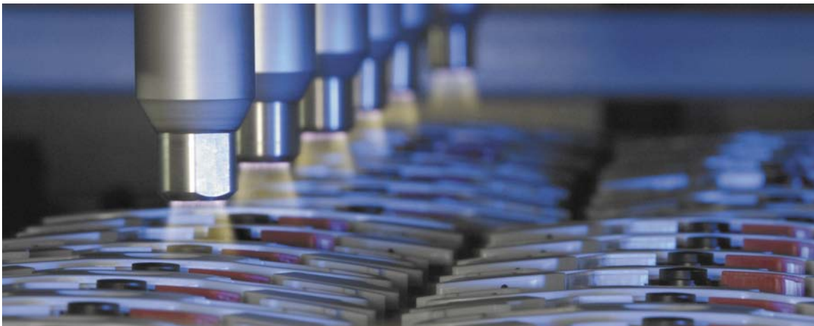
Six rotary plasma jets work in-line around the clock. Each week they clean and activate 180,000 visible parts made from PC and (PC+ABS) blend in a single step.
