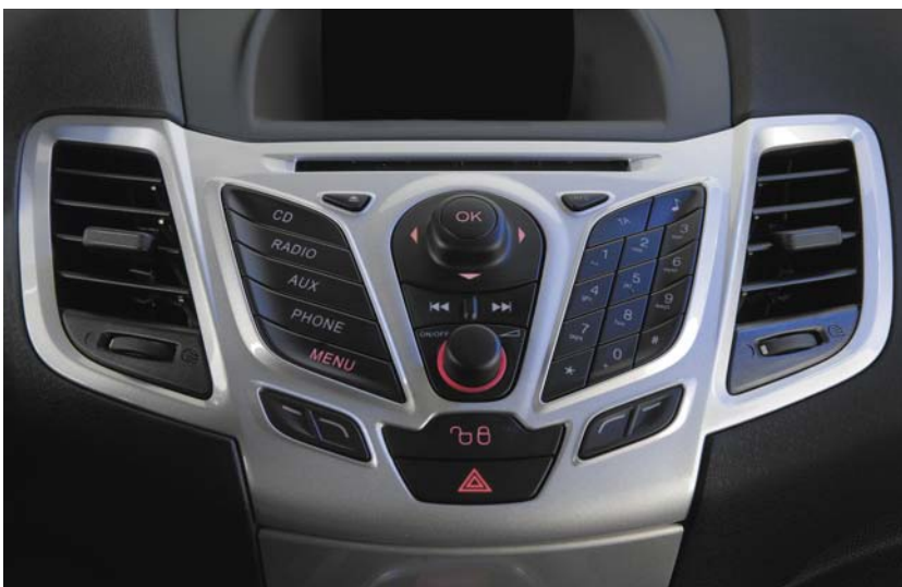
The integrated control panel (ICP) forms the centrepiece of the dashboard. The plastic switches are pretreated with atmospheric plasma before painting to ensure a flawless finish and an adhesion that will last for years.
