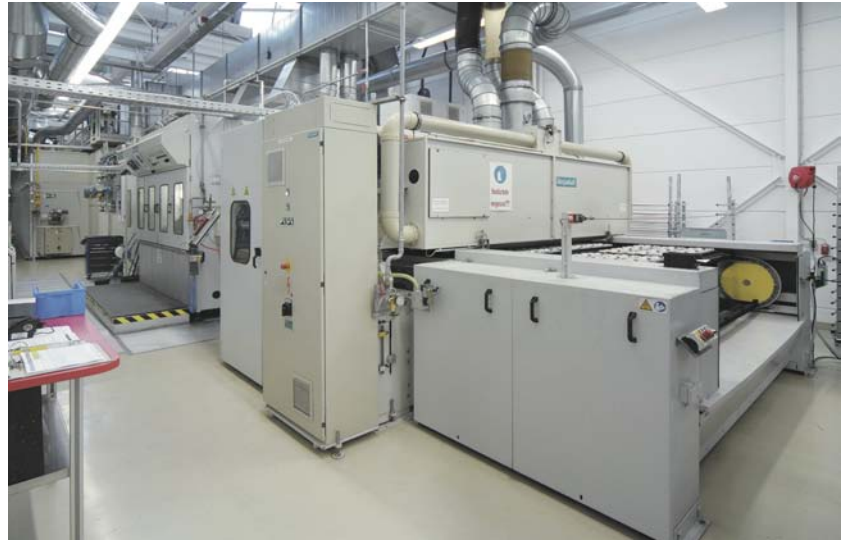
The «Openair» plasma system (3rd unit from the front) takes up only 1 m of a painting line with an overall length of 25 m
