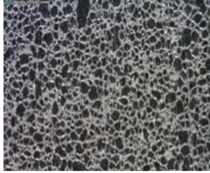
Fig. 5. The sintered UHMWPE structure of the ski base before treatment. Blockages and dust have accumulated in the micro-cavities (figure: Environment Park)
