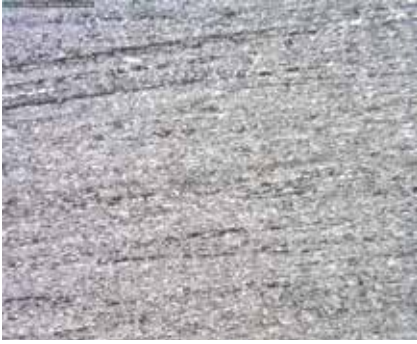
Fig. 4. Micro-cavities in the three-dimensional honeycomb structure of UHMWPE have collapsed: At this stage it is no longer possible to apply wax (figure: Environment Park)
