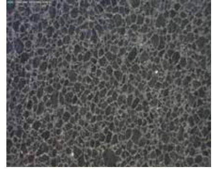
Fig. 6. Base structure after plasma treatment: The micro-cavities are clean and have expanded (figure: Environment Park)
