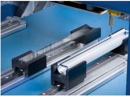
Figure 5 > Application of adhesive to the plasma-treated groove in the aluminum housing
